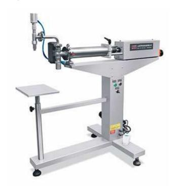
Liquid Paste Filling Machine is a volumetric piston filler, semi-automatic filling machine suitable for any kinds of liquid or low viscosity, the piston suck the material up, and then push it out in a certain quantity. We can adjust the sensor to adjust the route of the piston, to control the filling volume.
