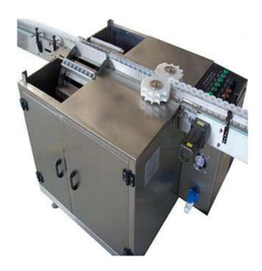
BXP-300 Automatic Bottle Rinse for the application of water and air rinsing to clean plastic or glass bottles before filling. The machine is composed by a short conveyor, bottle index wheel, water collect tank, bottle snap roller, water/air filter, water/air blowing system. The bottle loading/unloading through loading/ unloading turntable (alternative Ø 620mm or Ø 900mm), or directly from an production line.
