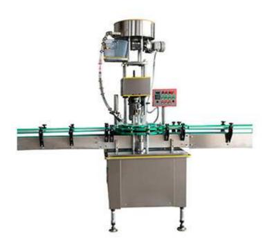
The automatic aluminum ROPP capping machine uses the automatic aluminum cap feeding and capping machine for the high-speed production line. It adopts the servo motor driven aluminum cap feeding and capping machine to sort, feed and locate caps with stable torque by one machine. It simplifies the arrangement of the production site. Rotary disks introduce bottles to the aluminum capping machine before locating and capping.
