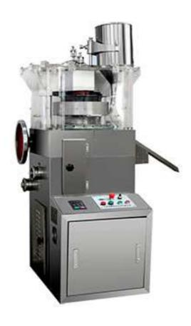
The machine is a latest rotary tablet press researched, developed and designed by our company, used to press granular raw materials into tablets of various shapes. In addition to making round tablets, it can also make special shaped tablets, special tablets, double-layer tablets and ring-shaped tablets, which can be customized according to your requirements. During the operation, the noise is low and the pressure is high, and the machine will stop in case of overpressure to avoid damage to it.
