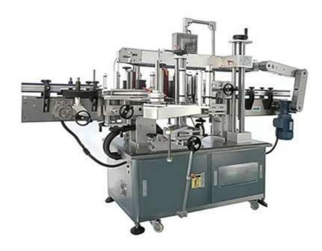
This machine is suitable for flat bottle, oval bottle, square bottle or irregular container, attaching two labels at the same time, and can select Single or double-sided stickers.
