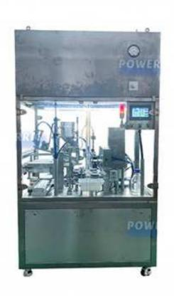
Put the syringe honeycomb on the special fetal membrane manually, and hang the syringe on the bottle comb plate together with the fetal membrane at one time, and then automatically enter the filling dial row by row from the slide. The dial rotates intermittently and feeds at a time. Insert a syringe into the dial wheel and turn it to the corresponding work station.
