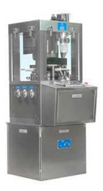
ZPS-20 rotary tablet press is a kind of intelligent small rotary tablet press. It is suitable for small batch production of pharmaceutical industry R & D centers and laboratories.
