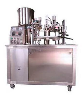
This machine applies the once transmission principle. It uses the slot wheel dividing system to drive the table to do intermittent movement. The machine has 8 sits. Expect manually putting the tubes on the machine, it can automatically fill the material into the tubes, heat both inside and outside of the tubes, seal the tubes, press the codes, and cut the tails and exit the finished tubes.
