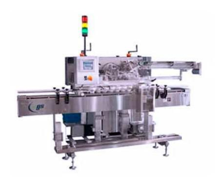
The MGS Machine Model TopSerter II™ has a solid reputation for handling your outserter applications. It will feed, glue, place and verify an outsert.
