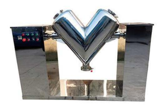
The mixing cylinder of V-type mixer is two asymmetrical cylinders, and the material is high quality stainless steel plate rolled round and tightly welded. The two ends of the cylinder are oval head, and the two heads are equipped with feeding ports, which is more conducive to the cleaning of the cylinder after the material is mixed. The inner and outer walls are polished and polished with smooth surface, no dead Angle, complete discharge, easy to clean and so on.
