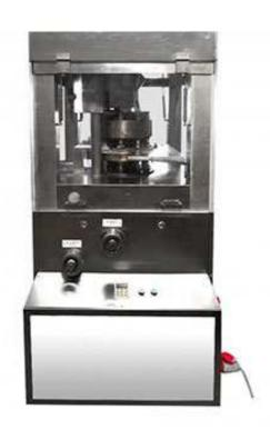
The technological process of tablet pressing machine includes overfilling, quantification, prepressing, main pressing forming, tablet production and other procedures. The upper die hole of the machine is loaded with the upper punch rod, the middle die is loaded with the middle die, and the lower die hole is loaded with the lower punch rod.
