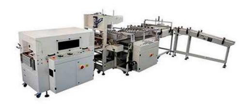
The combined Tower packaging machine ZF-XD450 uses an adjustable push plate to automatically arrange and automatically erect multiple rolls of tape to form a cylindrical packaging. The packaging speed can reach 12 barrels per minute. Suitable for multi-roll packaging of OPP sealing tape, stationery tape and PVC electrical tape.
