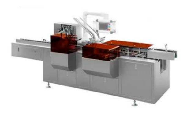
Automatic Cartoning Machine can pack products into carton box and seal the box automatically.
