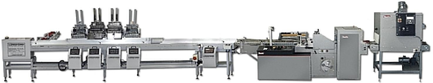
Collation, packaging of greeting cards and envelopes into boxes and shrink wrapping. Design/build a turnkey line that feeds, collates and shrinkwraps the box sets, inline rejects allow the line to run continuously, while rejecting any short packs.
