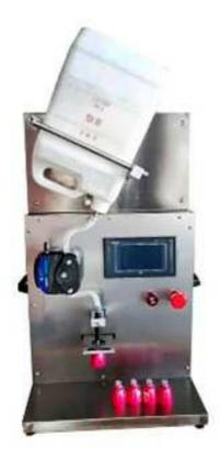
It can be applied to liquids, fluids, and washing products with different viscosities. The parts in contact with materials are all made of stainless steel, which has anti-rust and corrosion resistance. It is widely used in food, cosmetics, medicine, grease, daily chemicals, and washing. Filling products in various industries such as chemicals, pesticides, and chemicals. The linear filling method can be used for different types of solution filling.
