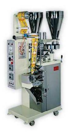
Vertical Form-Fill-Seal Machine SP-202D / SP-203D for packaging powder or granulated products such as coffee, condiment, dry vegetable. Two products can be metered separately mixed together and then packaged.
