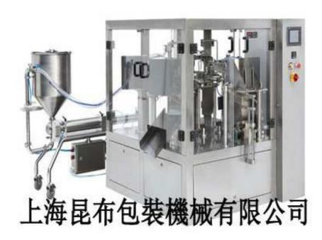
This device consists of a bag automatic packaging machines and liquid filling machine supporting body butter is made. Mainly applies to: detergents, yellow sprinkles, soy sauce, vinegar, juice, beverage, pot bottom material, ketchup, peanut butter, jam, chili sauce, bean paste and other materials, automatic weighing and packing.
