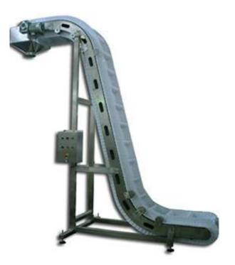
This kind of conveyor is used mainly to convey the solid food, such as rice, chip potato, candy, vegetable, etc. The conveyor is made of 304 stainless steel and plastic (PP), which is hygienic and healthy.
