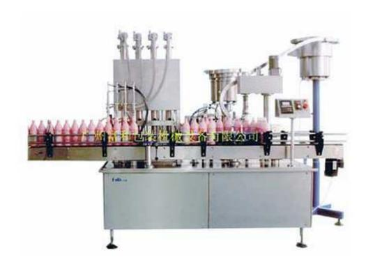
FHGF-4G series piston type, filling and sealing all-in-one machine, the structure is compact and high degree of automation, so it can have mass assembly line work in a small space. The filling system all adopts import pneumatic element FEST0, which the machine has powerful motive power and high reliability in filling different high viscosity liquid products. In the machine all the contact surface and corner piece with liquid, the roughness reach 0.5um, correspond GMP standard.
