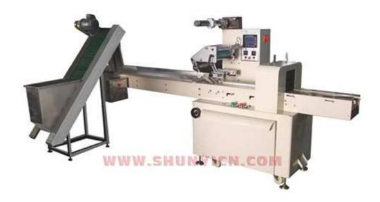
This machine adopts AC machine step-less speed regulation, with stable running and low noise. This machine has trademark positioning device, positioning is reliable.
