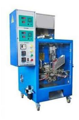
The machine is suitable for the vacuum package of granule material such as tea, meddler, etc.
