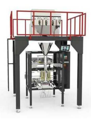
Suitable for granule type of products. The target weight is controlled by linear vibration units. With respect to product type and desired speed; 2 or 4 line types are available. The magnitude of vibration level for each line is adjustable. The accuracy of each filling is controlled by tuning each line vibration magnitude. The average accuracy is depending on product type.
