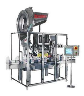
The NRX-4000 In-line Capping System is a breakthrough in machinery design. It is the first In-line capper to reach the 600 cap-per-minute speed, and has 18 patents approved by the US patent office. NRX-4000 comes equipped with our H-42 hopper/sorter or our HES bulk cap hopper/elevator/sorter depending on your needs. Also, new "gull wing" gripper design, touch screen controlled remote operator interface, 9'6" of conveyor, and adjustable "on the fly" air clutches are all standard.
