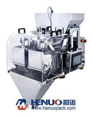
This kind of weigher is suitable for weighing small granules and powder, such as sugar, salt, seed, rice sesame, glutamate, coffee powder and seasoning powder, etc.
