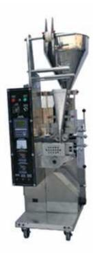
The machine is designed and manufactured specially for water, honey, oil, sauce, jam or similar liquid products. Driven by servomotor, the piston back and forth to fill liquid; furthermore, the filling range can be adjusted automatically through computer The processes of bag making, measuring, filling, sealing, cutting, counting and hot pressing codes can be done automatically. Packing material include several kinds of heat-seal lamination, such as PET/plated AL/PE, PET/PE, NYLON etc.
