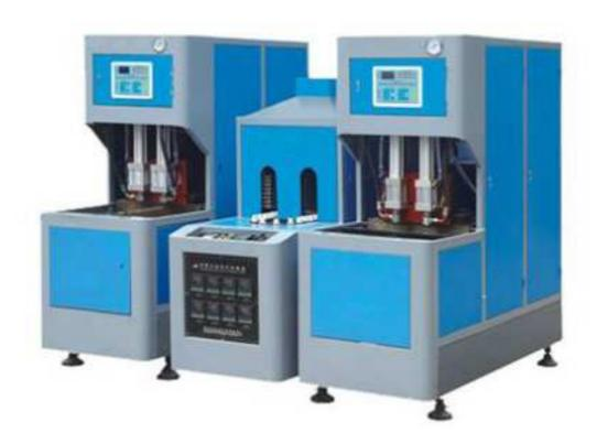
PET Plastic raw materials to make bottle embryo, and then blowing. The commonly used is the environmental protection plastic PET material. Using the machine to blow out of the wind, blowing PET plastic body attached to a certain shape of cavity, thus made products.
