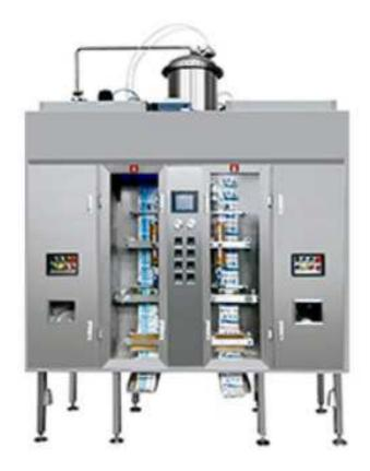
The machine applicable to pack liquid foods, such as milk, bean milk, peanut milk, juice, beverage, sauce and drinking water etc. packing automatic forming pouch, filling, sealing, counting printing date, UV sterilizing. SUS 304 material are used for sanitary warranty.
