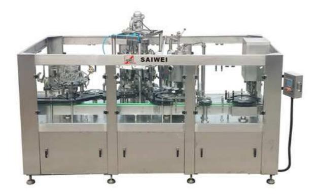
The machine has five parts: washer, pulp filer, juice filler, cap heat sealing or frequency sealing. The machine has two kinds of filling types, including bottle seated type and bottle neck clamping type.
