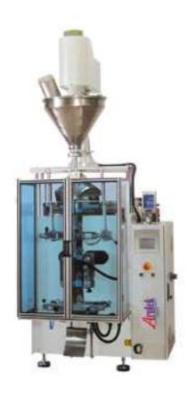
With this machine you can automatically fill powder (Cacao, 3in1 coffee, powder coffee, spices, vanilla, powder drinks, powder sugar) inside of packet with servo motor and auger system. And with this machine you can make quadro, pillow and standup pouch packs.
