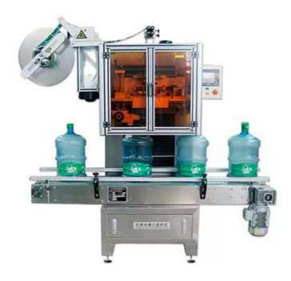
New Style Automatic Sleeve Labeling Machine with Steam Tunnel HTB-50 is suitable for different type of bottles. The machine mainfram is stainless steel, simple, safe maintenance and waterproof. And the spare part of machine adopts famous brand, long life span, so easy to repair and maintain, save time.
