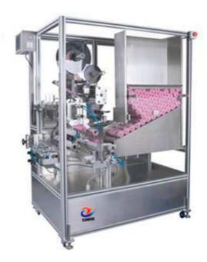
The Tube Labeling Machine can be an ideal facility that sticks a roll of self-adhesive paper labels to a PCB, product, or specified packaging. As an indispensable part of modern packaging, it has wide range of application, which can meet the full-round labeling or semi-circular labeling of round bottles. Compared with ordinary product on the market, it is simple to switch, and the adjustment is convenient.
