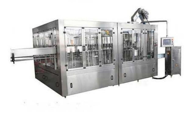
The CGF32-32-10 Bottled Water Filling Machine combined water bottle washing, filling and capping into 3 in 1 monoblack. It is suitable for both plastic polyester bottle (PET bottle) and glass bottle with screw caps for non-aerated carbon dioxide drinks such as mineral water, pure water, non-gas water, spring water and so on. The water filling machine design could shorten the time for the drink material contact with outside, increase the sanitation condition through economy benefit.
