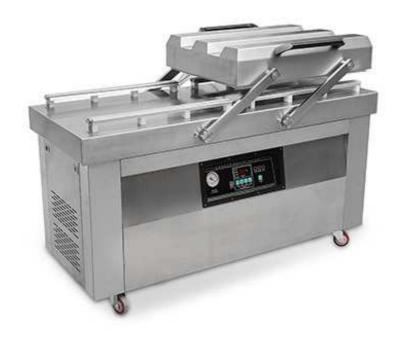
DZ-600/2SA double chambers vacuum packer can finish the whole programs of vacuum extraction, gas injection (optional),sealing, cooling and exhaust automatically. The products after packing can be prevented from oxidation, going mould, insects or getting damp, thus can be kept fresh for longer time. This is an efficient, sustainable double chambers model for outstanding vacuum packaging results.
