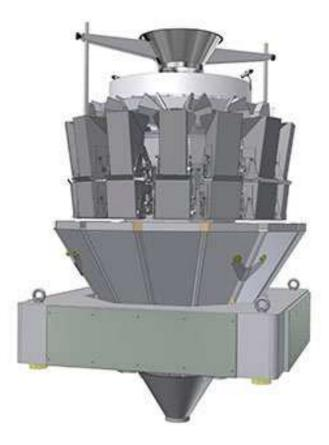
Anti-sticking Screw Feeding Multihead Weigher is well known for its pointier chute, which make pruducts drop faster, also with independent chutes, the products won't bump to each other.
