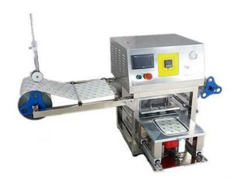
Automatic plastic food container tray sealing machine is a desktop pneumatic type sealing machine, suit for sealing PP/PET/PS/PVC...trays, rectangular, square or round kinds tray.
