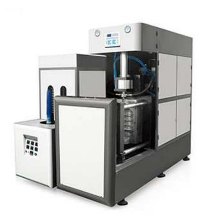
WBS-1-20 Semi-automatic blow molding machine blows PET bottle from 10L-20L. neck size from 45mm-200mm. Also can do the lamp cover.
