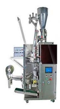
The equipment is controlled by PLC, driven by servo motor and sealed by ultrasonic. Suitable for tea bagging, coffee, Chinese herbal medicine, scented tea, etc.
