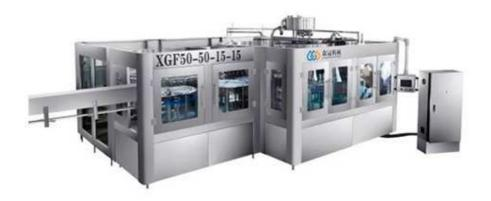
This machine works harmoniously with air-conveyor belt, It holds the bottles by the neck, thus, reducing the possibility of bottles falling over during conveying process. This machine is used to fill still water into pet bottle and with screw caps capping function.
