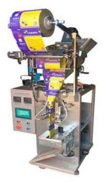
The three sides sealing powder filling packing machine can automatically complete all the work in the packaging process, such as measuring, bag-making, filling, sealing, printing date, cutting, counting, cutting and tearing easily.
