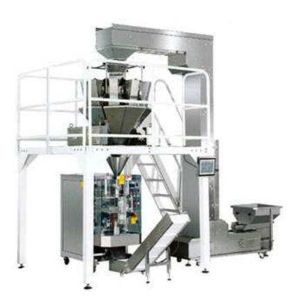
The bagging machine is widely used for packing of products in shape of granules, stripes, slices such as candy, potato chips, jelly, and peanuts.
