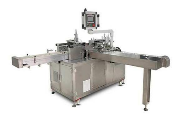
The machine replaces the manual packing, the operator as long as it will be a bag, a one-time will take a bag of hundreds of bag in the equipment, equipment of manipulator automatically get bags, date printing, open bag mouth, push products, exhaust, sealing, output.
