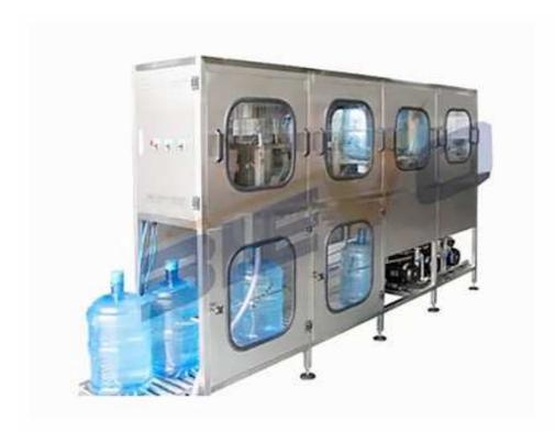
The machine is used for 3 gallon & 5 gallon water filling, which is composed of washer, filling and capper.
