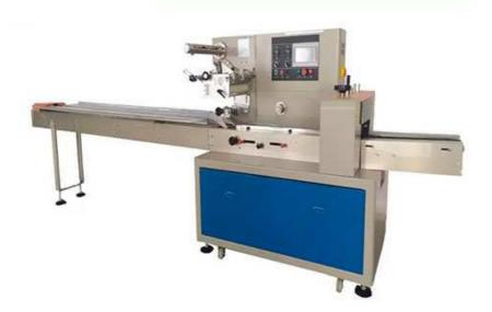
Horizontal flow wrap machine is ideal for suppliers of products that must be packaged individually. Flow wrapping is a horizontal packaging process in which product enters the machinery and is wrapped in clear or printed film. The result is a tightly fitted flexible package with a horizontal back seal and end seal.
