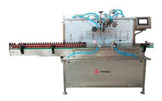
The PLC Based Filling Machine is compact and highly efficient machine with elegant look. This multi-functional multi featured machine meets the GMP requirements of filling for glass & plastic bottles. The flow of liquid is measured and converted in to electronic signals being controlled by microcomputer base circuitry. Minimum adjustment required to set different capacities of containers. The entire range can be set on the same machine without any change parts with help of servo system.
