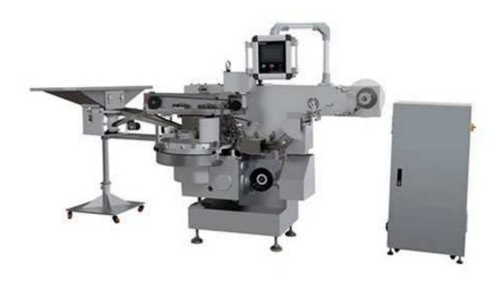
The SL-SBQS450 series of peanut-shaped chocolate wrapping machines are wrapped in pure aluminum foil wrapping paper. The wrapping film fits perfectly into the chocolate and reveals the shape of the peanuts.
