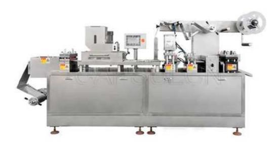
Flat-plate blister packaging machine is a kind of special equipment for PTP/PVC or PTP/PTP compound sealing packaging of drugs (including tablets, capsules and ampoules), food, medical instruments and similar materials. Due to positive pressure forming, flat pressing heat sealing, the finished blister sheets are even and smooth, which makes this machine favored by the whole industry.
