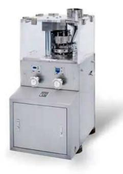
The electric rotary tablet press machine ZP-9B enhanced type is a single press type automatic rotary continuous tablet press machine used for the compression of special-shaped and round tablets, which is suitable for laboratory, small-scale product processing or small-scale production industries, etc.
