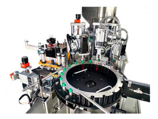
Suitable for vertical labeling of testing tube containers for the pharmaceutical industry, star wheel driving ensures high speed and high precision, and is capable of labeling full or half round.
