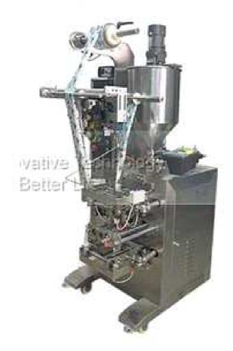
This Instant Noodle Sauce Packing Machine adopts correcting system controlled by microcomputer, owing to a response signal is and set pass through microcomputer it can accomplish whole set to synchronization, sack length,position fixing, voluntarily follow the tracks of light-mark and voluntarily diagnose trouble and show to screen.
