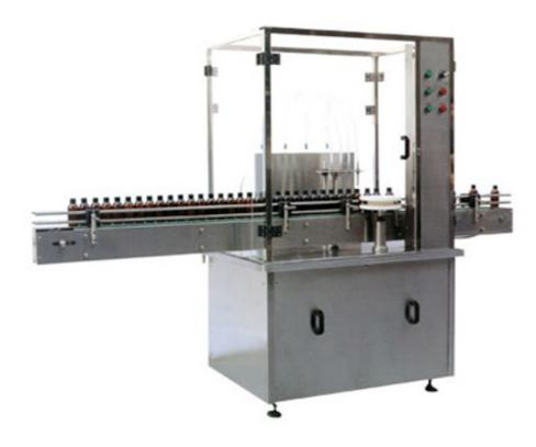
This machine is applied to fill liquid in the pharmacy, food, chemistry and agriculture, etc. It adopt piston-measuring pump to fill straight for bottles with different sizes and materials. It has the advantages of compact and reasonable structure and simple operation. Customers may choose to purchase dustproof cover.
